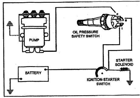
Wires should be 18 gauge insulated, or heavier and routed so as to protect them from exhaust heat and anchored securely at frequent intervals to prevent chafing.
